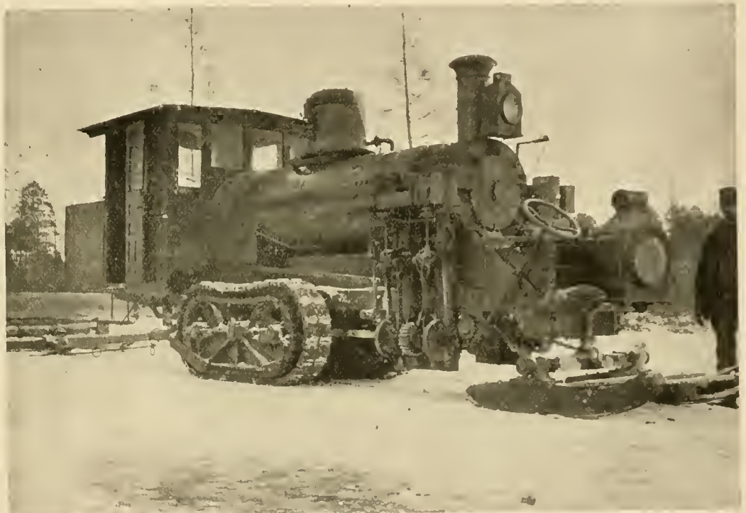
STEAM LOG HAULER IN USE ON THE FORMER CHIPPEWA INDIAN RESERVATION IN MINNESOTA.
